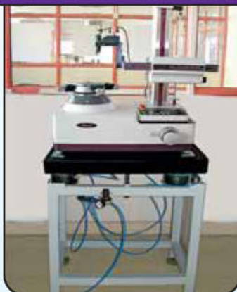
Mitutoyo Roundtest RA 1600 installed on Dynemech Anti Vibration Table DIT-AL-02
