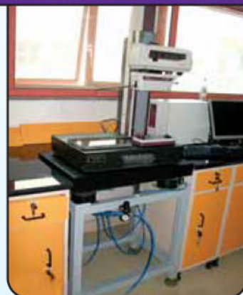
Mitutoyo Contracer CV-3200 installed on Dynemech Anti Vibration Table DIT-AL-02
