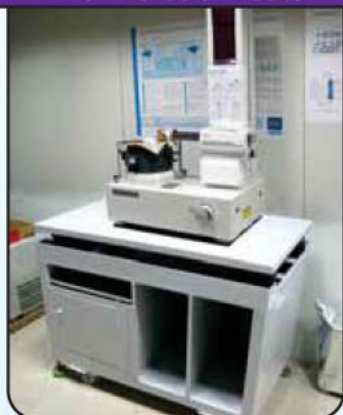
Mitutoyo Roundness Tester RA 2200 with LC-0.13nm installed on Anti-Vibration Table
