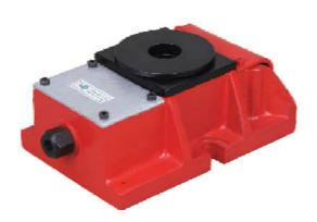
VHS Festofix Leveling Wedge Mounts are useful in leveling and aligning machinery to very strict tolerances and make it possible to vary adjustments at any time, even under maximum loads requiring only a small hand wrench to adjust. These mounts provide the most rigid machine to foundation connection. The 3 piece wedge design provides true vertical lift and eliminates lateral movement as machines are raised or lowered.
