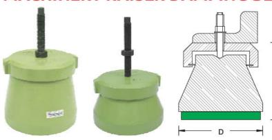
**Series DRC** are suitable for machines having plain hole in the base. Levelling is done by turning the bolt which lifts the cover plate along with the machine. Available both in 150 &100 mm height.
