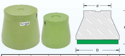
**DYNEMECH** Series DR, are suitable for machines having tapped hole in the base. The bolt rests over the dimple provided on the top face of the mount. Dimple size is provided as per the bolt diameter in the machine base.
